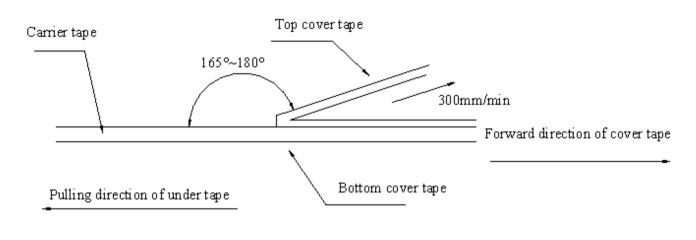
\*\*\* In the case, the cover tape is pulled off under the above conditions, the cover tape adhesion strength should be 10.2g~71.4g Plastic tape:10.2g~71.4g
