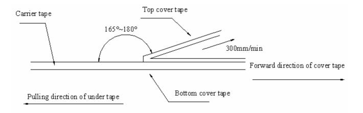
\*\*\* In the case, the cover tape is pulled off under the above conditions, the cover tape adhesion strength should be 10.2g~71.4g Plastic tape: 10.2g~71.4g
