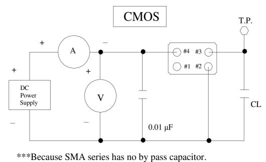
So, we recommend our customer to use capacitor  $0.01 \ \mu\text{F}$  in join Vcc and GND.
