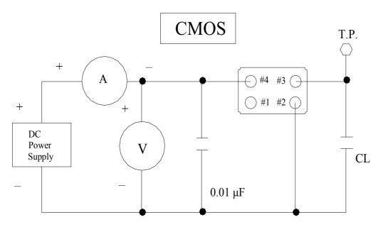
\*\*\*Because SMA series has no by pass capacitor. So,we recommend our customer to use capacitor  $0.01~\mu F$  in join Vcc and GND.
